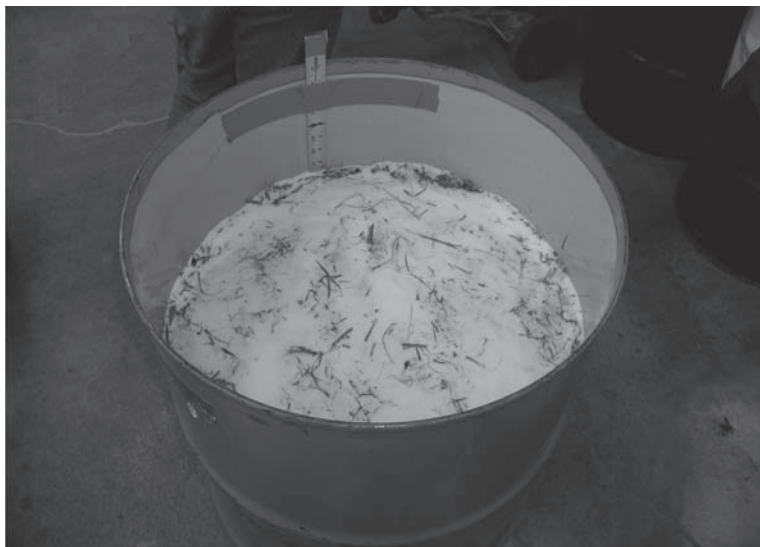
Figure 2. Salt cover illustrating amount of salt (1 lb/ft 2 ) added and change in height.
