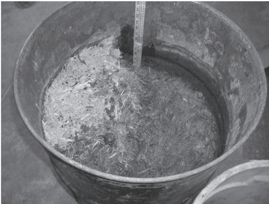
Figure 1. Picture of Control (uncovered) barrels depicting spoilage layer, fresh layer, and markings for determining the height of spoilage.
