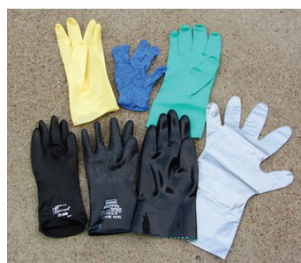
Figure 4. Chemical-resistant gloves (top row, left to right): natural rubber, disposable nitrile, reusable nitrile; and (bottom row, left to right) neoprene, butyl rubber, Viton, and barrier laminate.
