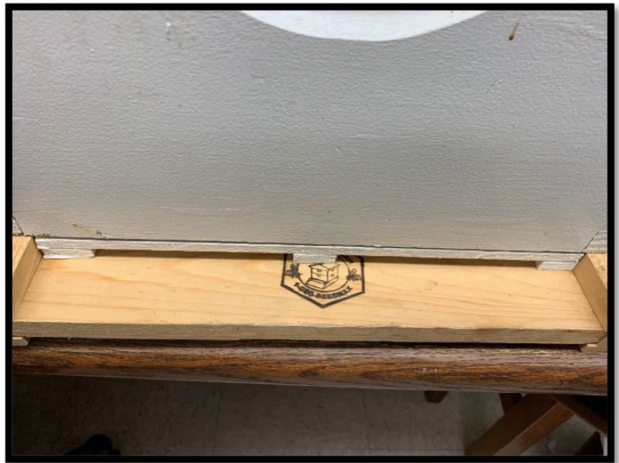
Figure 13. Place the hive box on top of the ASMG prior to nailing to ensure the ASMG is flush with the front of the box. (Photo credit: Sheldon Brummel).
