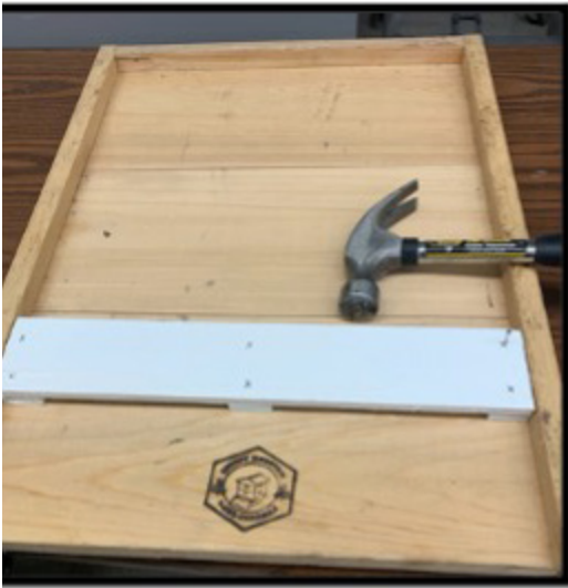
Figure 12. Place the long section on top of the spacers and nail where the “x” is marked. (Photo credit: Sheldon Brummel).
