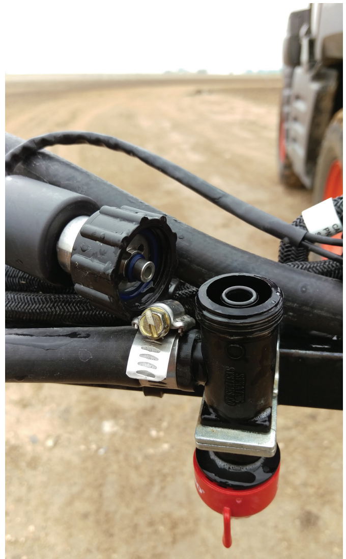
Figure 1. Solenoid valve equipped on PWM sprayer.
