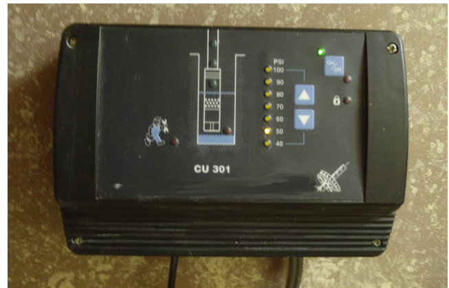
Figure 3. Control unit for a VFD system.
