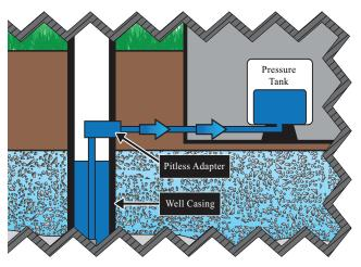
Figure 1. Water is pumped from the well through the pitless adapter to the pressure tank, then to various water fixtures in the building.
