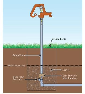
Figure 6. Pitless units reduce the risk of contamination from runoff
