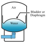
Figure 5. Diaphragm or bladder-type pressure tank.
