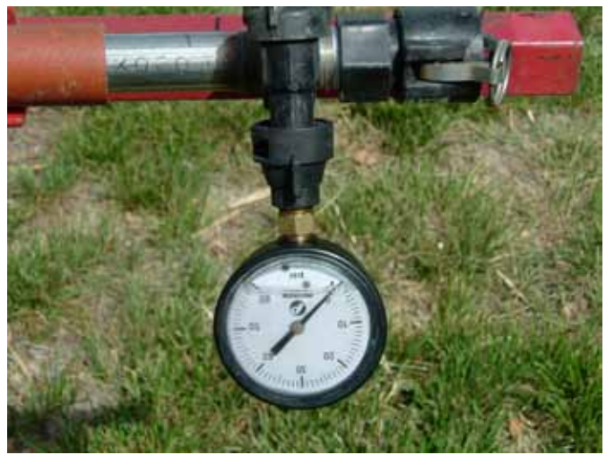
Figure 10. Gauge to check spray pressure on a wet boom.
