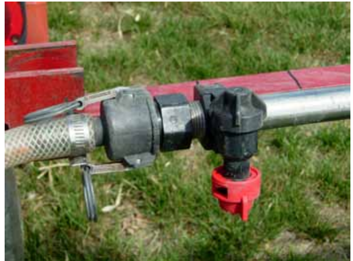
Figure 6. How wet boom is fed.
