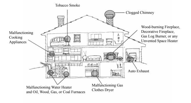
they can be overcome by other air movements, such as those created by bathroom exhaust fans, clothes dryers, air leaks in the house, and wind direction. High winds around the outside of the building or too short a chimney can create a downdraft. This occurs when a vent fills with cooler air that tends to fall, and the vent continues to be filled with more outside cold air, resulting in backdrafting.
