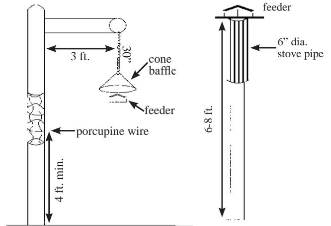
**Figure 3.** Two designs for squirrel-resistant bird feeders.
