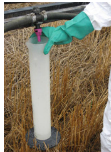
Figure 2. In a stationary position and with proper boom pressure, measure the output over the same time period used for the run. The number of ounces collected is equal to the gallons per acre.
