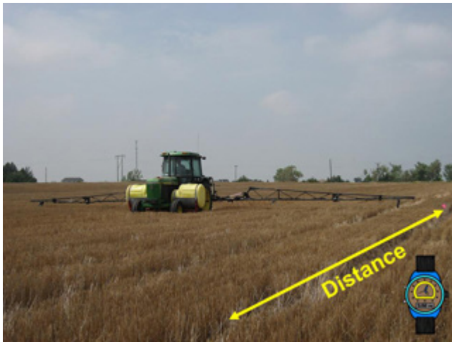
Figure 1. Measure the appropriate length for the nozzle spacing, then measure the time to run the course.
