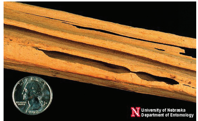
Figure 4. Smooth galleries of a carpenter ant colony in structural lumber. (Photo credit: James Kalisch).
