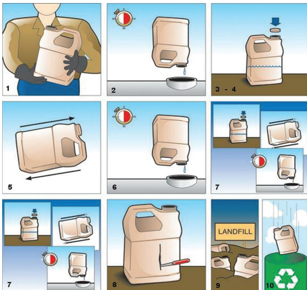
Figure 1. Triple-rinsing procedure for plastic pesticide containers. Used with permission from Fred Whitford, Purdue University. Scott Dallas and John Metzinger, illustrators.
