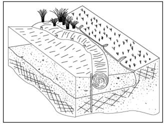
Figure 3. Coir fascines stabilize banks and help establishment of wetland plants. The coconut fiber accumulates sediment and biodegrades as plant roots develop and become a stabilizing system. (From Bestmann-Green Systems)
