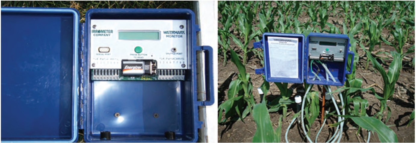
Figure 6. Watermark Monitor data logger. Up to eight Watermark sensors can be connected to the data logger to monitor matric potential continuously.
