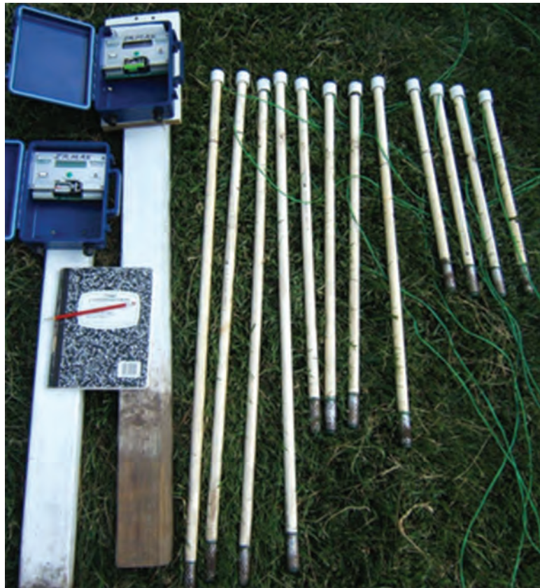
Figure 3. Watermark sensors attached to PVC pipes to be installed at different depths.
