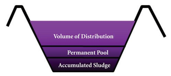
Figure 5. Stratification and design allocation of storage capacity in an anaerobic lagoon.
