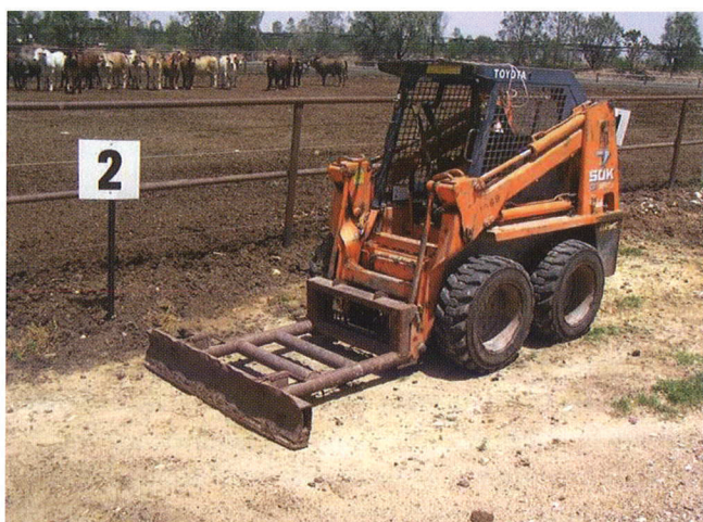
Figure 8. Skid steer loader fitted with attachment for cleaning fence lines.
