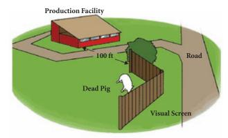
Figure 1. Carcass storage area for rendering pick up.
