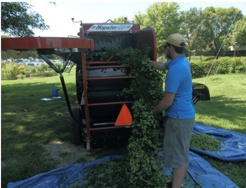
Figure 2. Mature hops are pulled through a harvester to remove all vegetation from the bine and through a series of incline belts and a blower, cones are separated from leaf litter.
