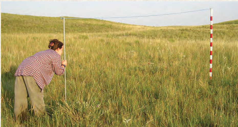
FIGURE 3. The proper use of a Robel Pole to measure Visual Obstruction Reading (VOR), a measure of cover density and biomass. Photo by Silka Kempema.
