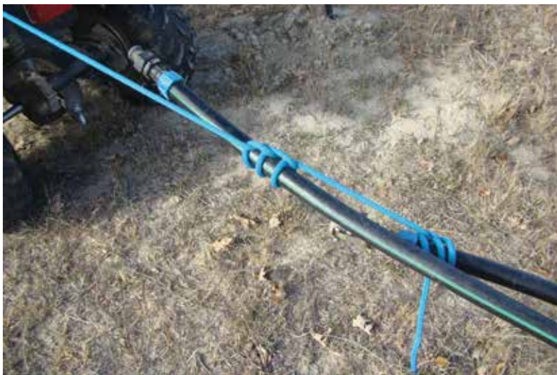
Figure 17. Securing tubing with a tow rope and clove hitches. Photo credit Jason Gross.
