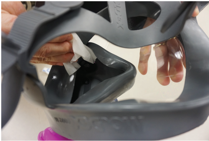
Figure 12. Dry with a lint-free cloth.
