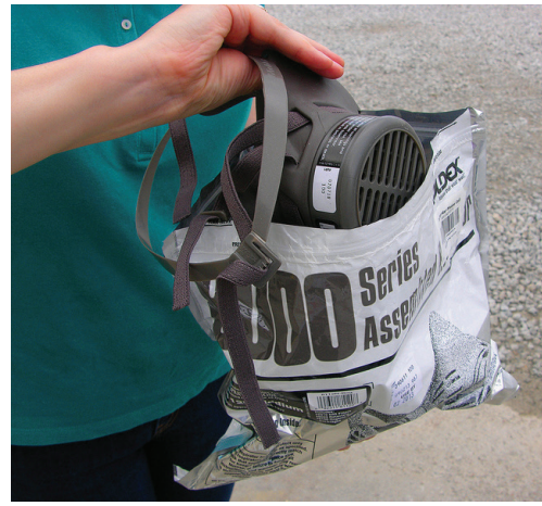
Figure 13. Store the respirator in packaging that can be sealed tightly. UNL photo.
