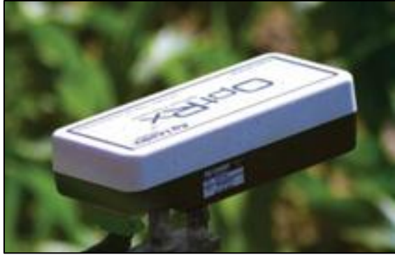
Figure 2: Active crop canopy sensor positioned over corn canopy.
