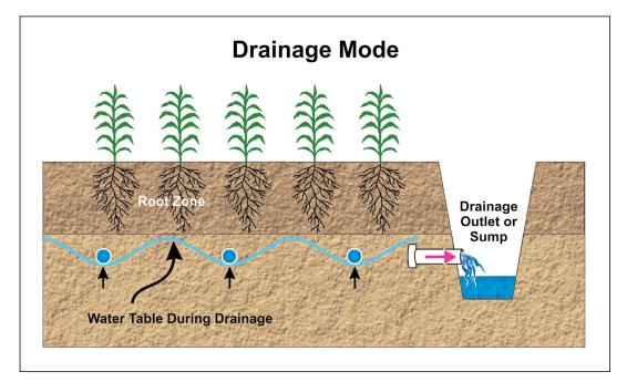
Figure 8b: Basic components of subirrigation system that is operated in a drainage mode. (Adopted from Brown et al., 1997).
