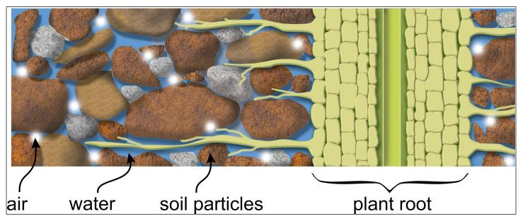
Figure 6: Soil structure components that influence soil matric potential value, in addition to soil water content.
