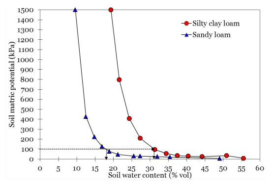
Figure 7: Example of soil-water retention curve for silty clay loam and sandy loam soils (example developed using Soil Water Characteristics/Hydraulic Properties Calculator developed by K.E. Saxton and W.J. Rawls, 2006).
