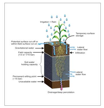
Figure 3: Schematic representation of some of the main soil-water, hydrologic, and related variables in a typical agricultural soil profile.
