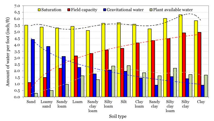
Figure 4: Amount of water (inch per foot) at saturation, field capacity, and the amount of temporary gravitational water [values are calculated using procedures outlined by Saxton et al. (1986) and Saxton and Rawls (2006)].
