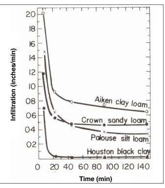
Figure 5: Infiltration rate as a function of time for various soil types (from Free et al., 1940).
