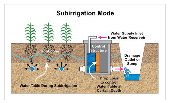
Figure 8a: Basic components of subirrigation system that is operated in a subirrigation mode. (Adopted from Brown et al., 1997).
