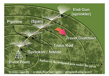
Figure 1: Some of the basic components of a center pivot irrigation system in the field.
