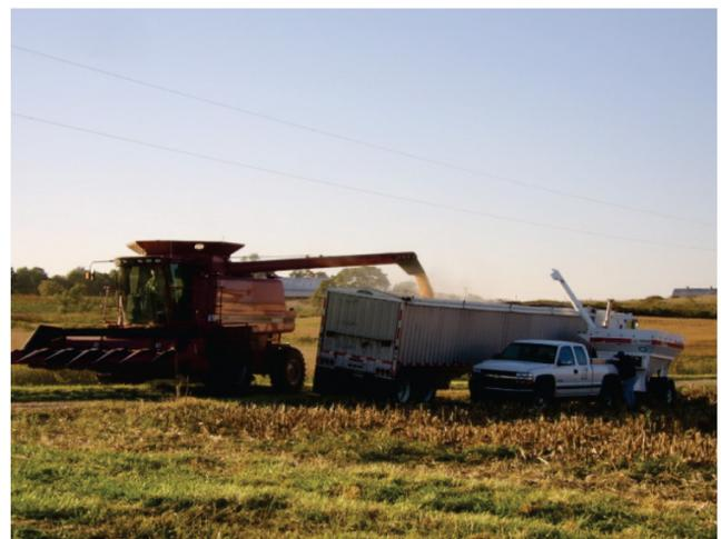
**Figure 2.** A grain cart equipped with scales or a weigh wagon is often used to quickly weigh loads for the mass flow sensor calibration procedure.
