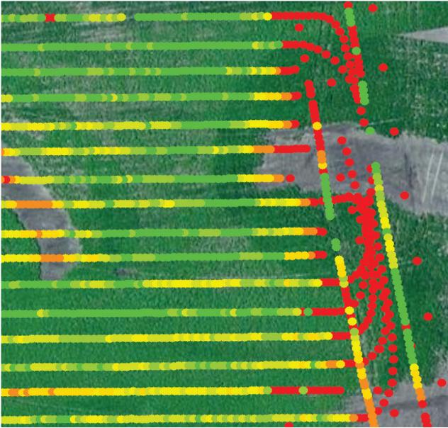
**Figure 6. Yield data points collected during turning in the headlands; points (in red) collected in the turn contribute to errors in overall yield estimates and representation within yield maps.**
