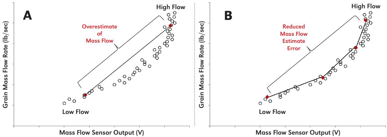
Figure 3. Potential error when using a two-point calibration (A) versus additional point (B). Calibration load points are shown in red.
