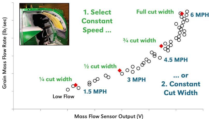
Figure 4. Two methods for varying clean grain elevator flow for mass flow sensor calibration: method 1, constant speed in green; method 2, constant cut width in blue. Calibration loads shown by points in red.
