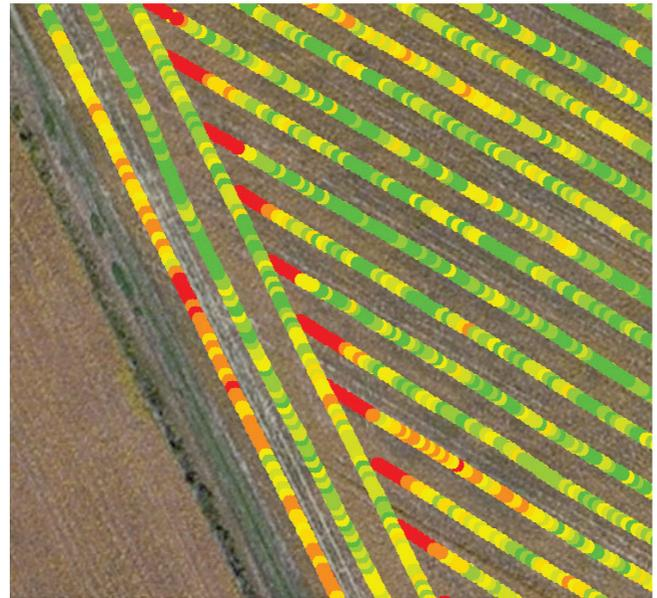
**Figure 7. Cut width errors contributed to lower yield data estimates within point row locations.**
