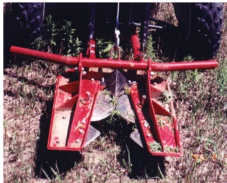
Figure 5. An ATV-mounted “cedar eater”.
