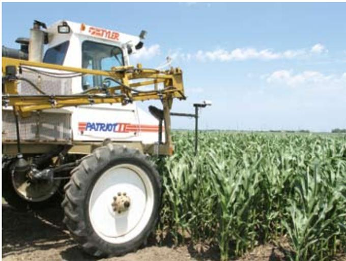
Figure 6. Active crop canopy sensor mounted on fertilizer applicator.
