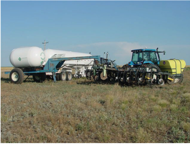
Figure 1. Applicator for dual application of ammonia and 10-34-0.
