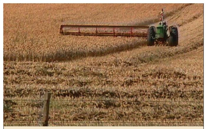
To prevent grain loss due to shattering, proso is often swathed and placed in a windrow when the top half of the head is ripe. Several days later, a combine with a pick-up attachment is used to harvest the grain.
