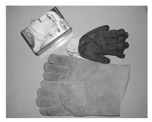
Figure 2. Top left and moving clockwise: Latex gloves, rubberized cloth gloves, and welder's gloves. Photo by Stephen M. Vantassel
