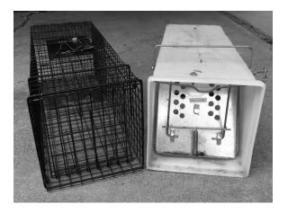
Figure 7. Cage traps have wire-mesh walls (left) while box traps (right) have solid walls. Photo by Stephen M. Vantassel.
