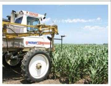
Figure 6. Active crop canopy sensor mounted on fertilizer applicator.
