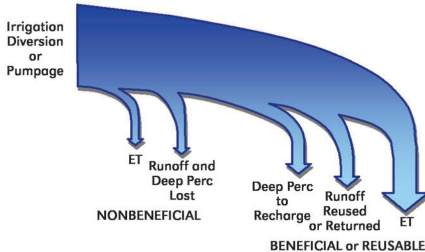
**Figure H-6.** Schematic drawing of the possible fate of water used for irrigation.
