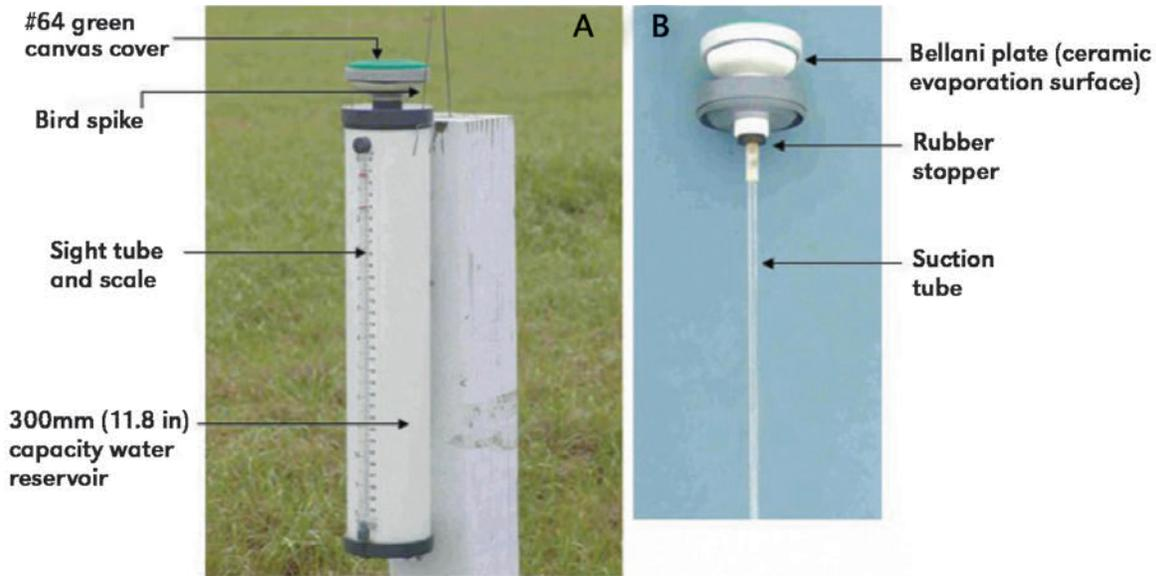
**Figure I-8.** ETgage used to estimate reference crop ET.
