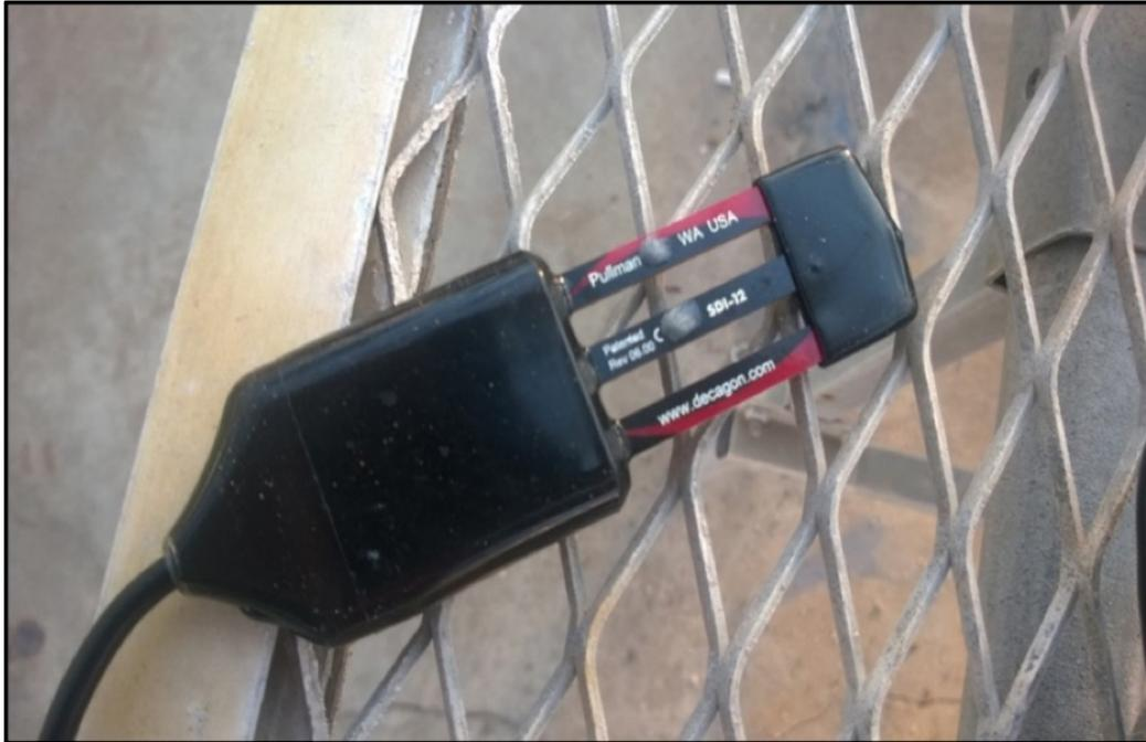
Figure 8. The 5TE frequency-domain reflectometry (FDR)-based soil moisture sensor from Decagon Devices Inc. (now METER Group Inc., USA), Pullman, Washington. The device measures volumetric SWC.
