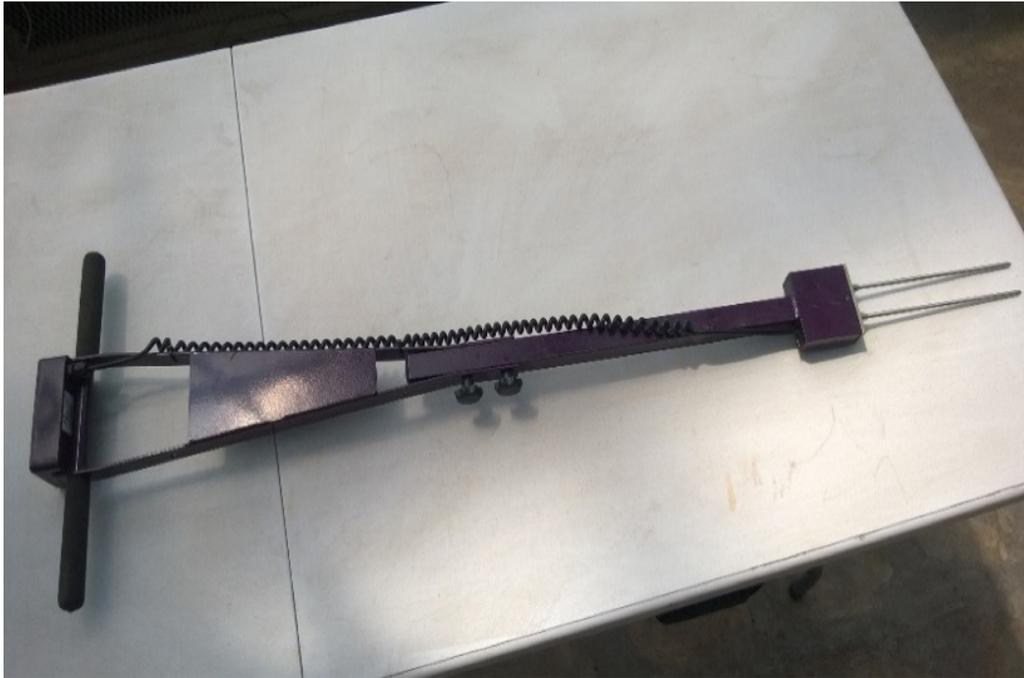
Figure 6. TDR 300 (FieldScout soil moisture meter, Spectrum Technologies) that measures volumetric SWC.
