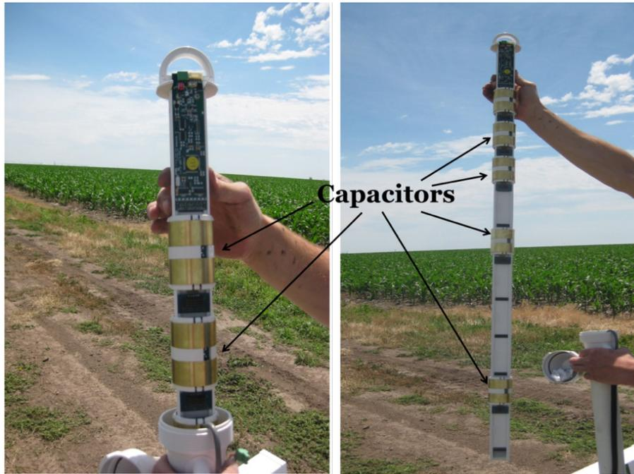
Figure 9. An example of a John Deere Field Connect™ capacitance-based soil moisture sensor used by the Irmak Research Laboratory at UNL's South Central Agricultural Laboratory. These sensors allow remote (telemetry) programming, measurements, and data downloading.
