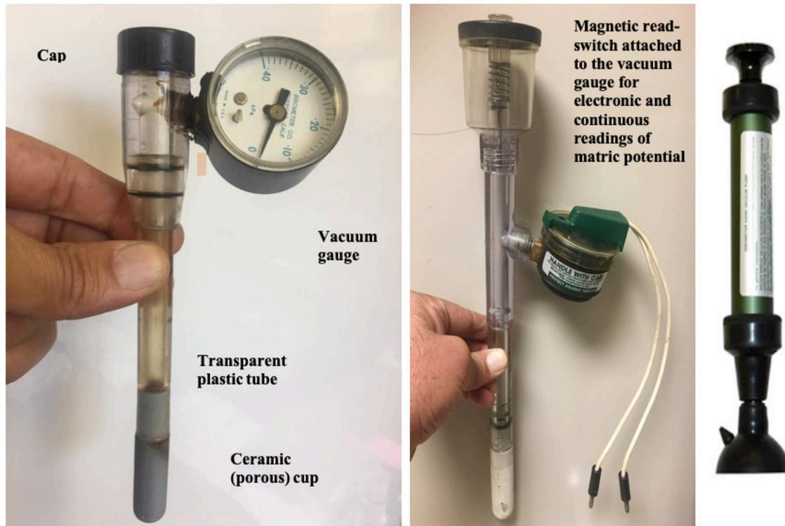
Figure 11. Tensiometer for soil-matric potential measurements and its basic components (left), tensiometer with a magnetic read-switch attached for automated control (middle), and a hand-held vacuum pump used to remove air bubbles from the tensiometer (right).
