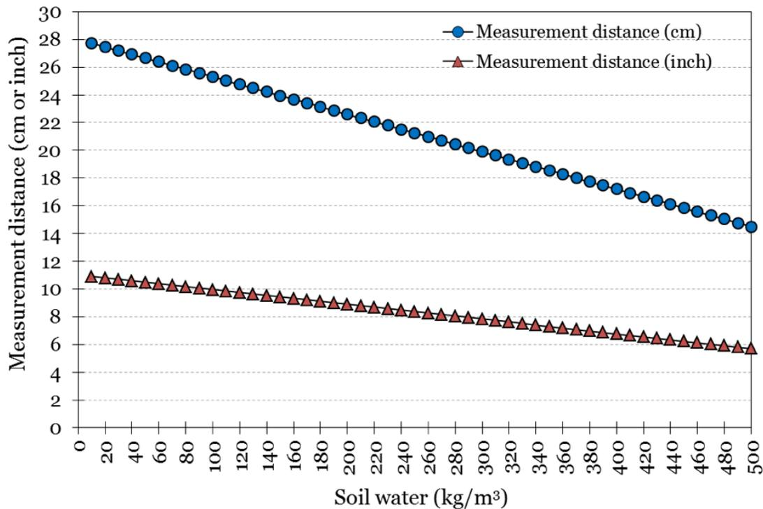
Figure 4. Relationship between the measurement distance (radius or area of influence) of the neutron probe measurements as a function of soil-water ( $500 \text{ kg/m}^3 = 0.02 \text{ lb/in}^3$ ).
