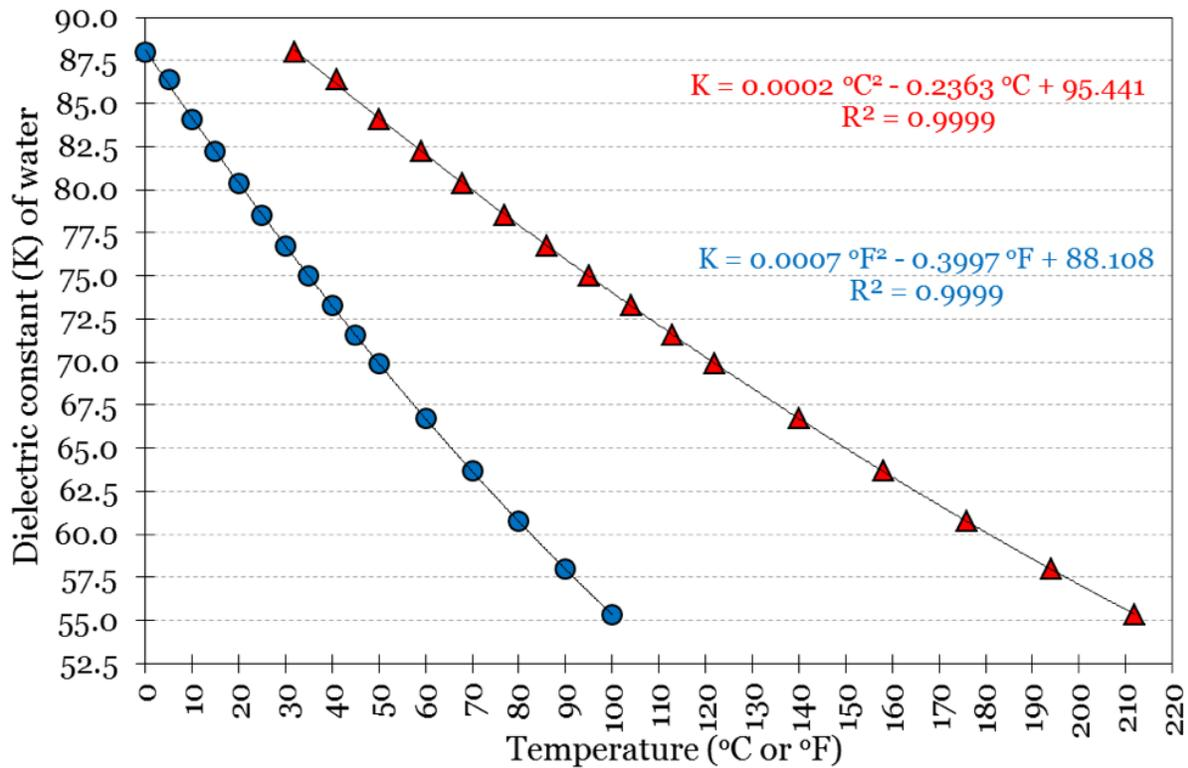
Figure 7. Relationship between temperature and dielectric constant of water.
