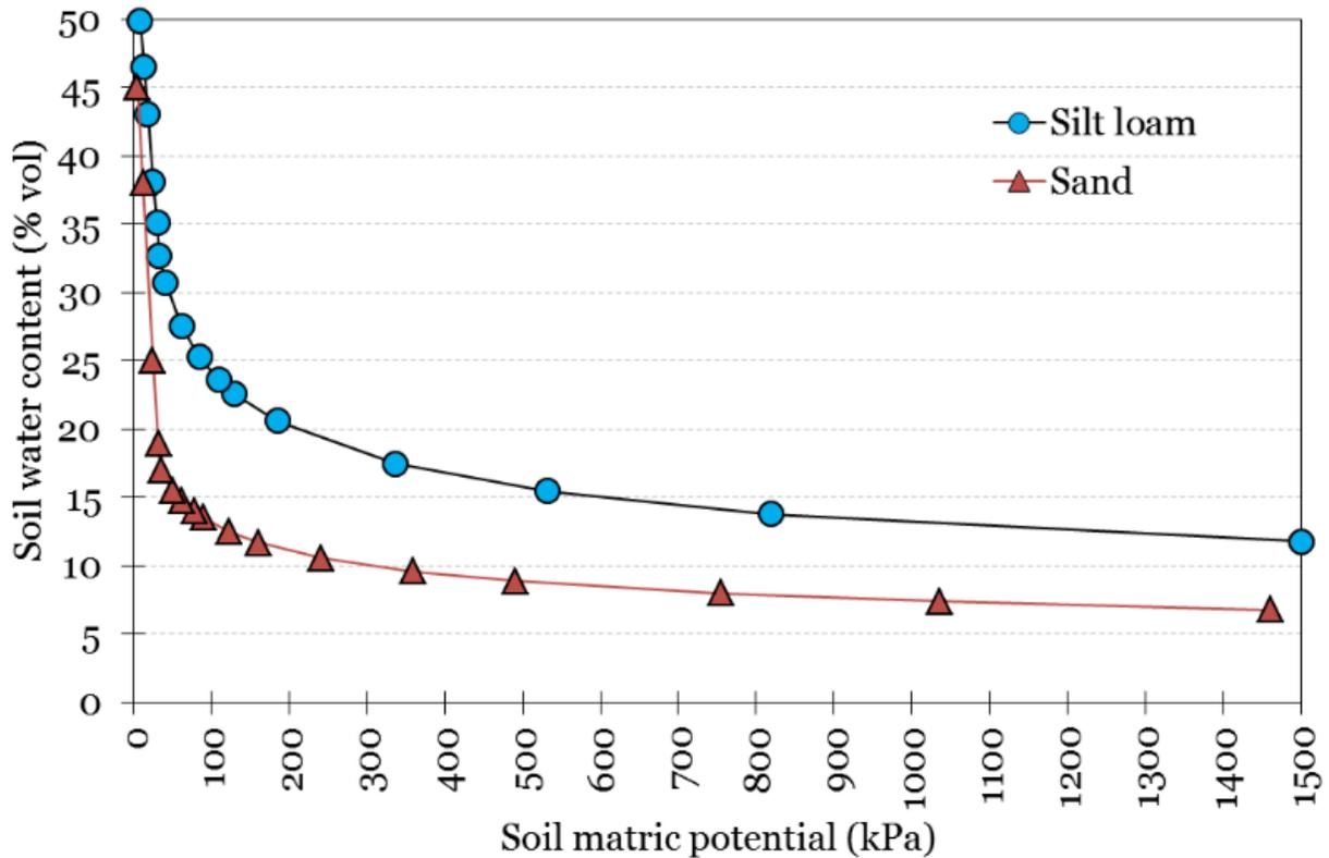
Figure 1. Relationship between SMP and SWC (soil-water retention curves) for two different soil types.
