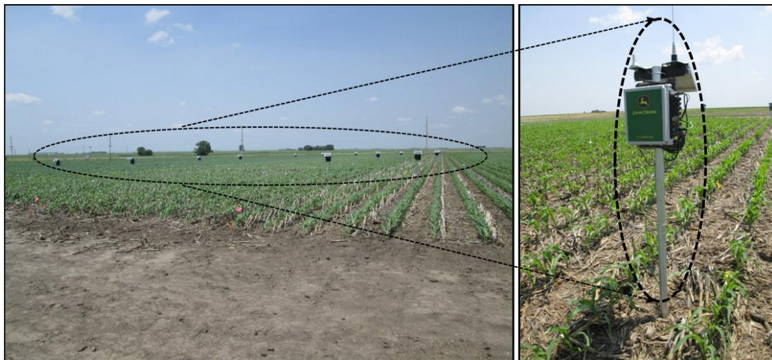
Figure 10. Example of John Deere Field Connect™ capacitance-based soil moisture sensors that are deployed grid-wise in a center-pivot irrigated maize field for research to investigate the spatial and temporal variability in soil moisture in the Irmak Research Laboratory at the South Central Agricultural Laboratory.
