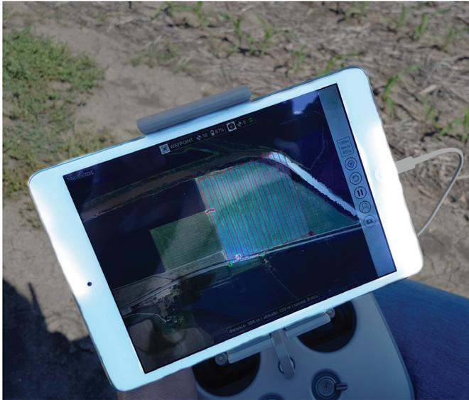
Figure 6. Images of a remote controller with flight planning software for systematically flying the field in a serpentine pattern.
