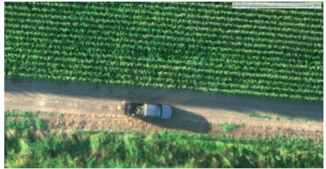
Figure 7. Example of imagery resolution obtained using a 5 band multispectral camera at 400-foot altitude. Resolution is approximately 3.5 inches per pixel. The pickup truck in the lower portion of the image allows for conceptualization of the image resolution.
