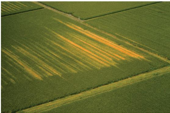
Figure 14. Aerial natural color images of a furrow irrigated field where water was not being uniformly distributed.
