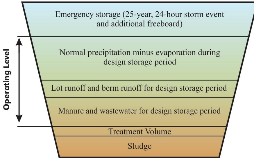
**Figure 2. Anaerobic treatment lagoon schematic showing volume fractions.**
