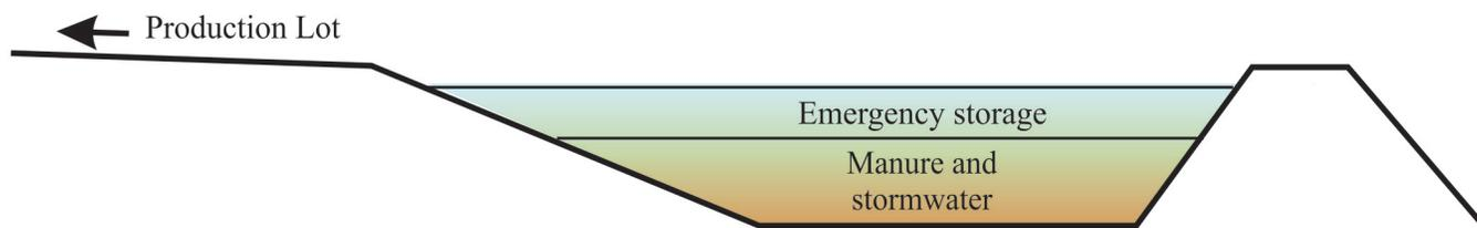
Figure 4. Runoff holding pond schematic showing volume fractions.
