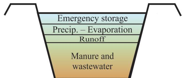
**Figure 3. Earthen manure slurry storage basin schematic showing volume fractions.**
