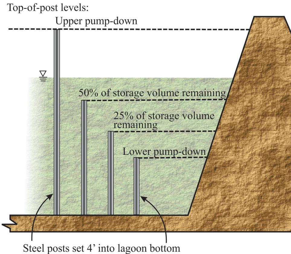
**Figure 10. Pump-down markers in an earthen manure storage can be a single post with graduations (a) (adapted from Pfoest et al., 2007) or a series of posts set at graduated depths (b).**
