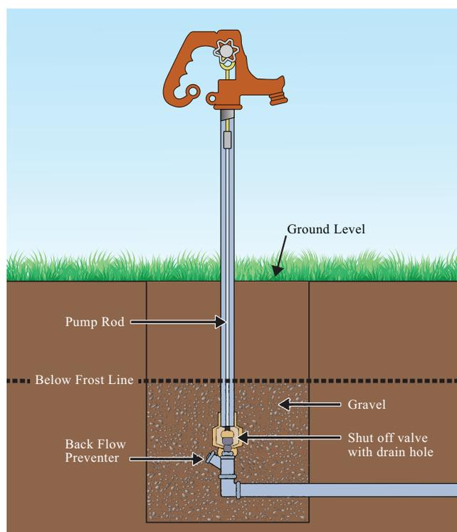
**Figure 6. Pitless units reduce the risk of contamination from runoff**
