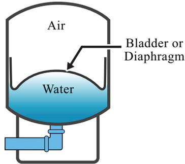
Figure 5. Diaphragm or bladder-type pressure tank.
