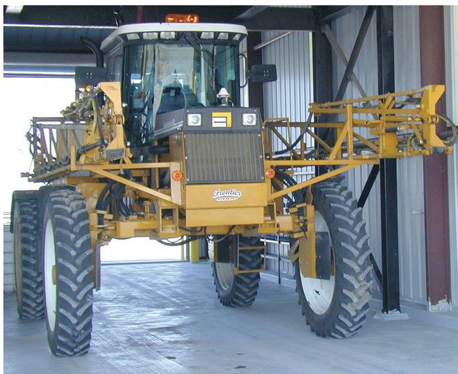
Fig. 1. Agricultural field sprayer for pesticide applications.
