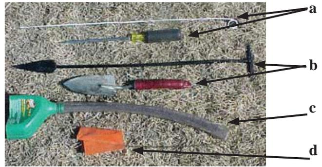
**Figure 5.** Tools for trapping or dispensing baits for pocket gophers: a) two-foot length of stiff wire or a long-handled screwdriver for probing, b) long-handled spade or spoon or a hand trowel for digging, c) a funnel for dispensing bait, and d) a flag for marking mounds. (Photo by Dallas Virchow)
