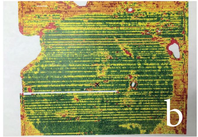
Figure 2a and 2b. Crop yield before (a) and after VRI technology (b). Figure a (left) has large areas of low yield represented by the white areas while Figure b has a more uniform yield map.
