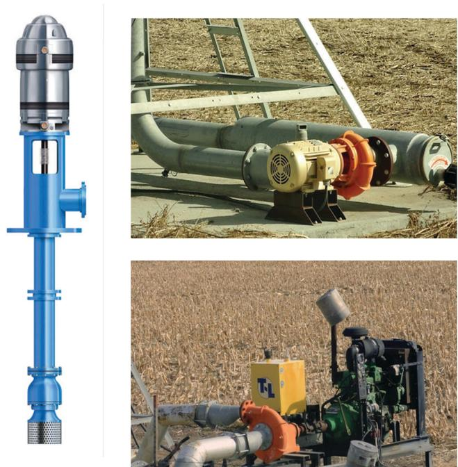
Figure 75. Examples of direct drives for motors and engines (drawing is courtesy of ITT Gould Pumps).
