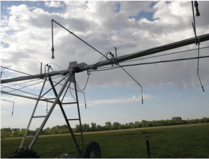
Figure 56. Center pivot equipped with boom backs.
