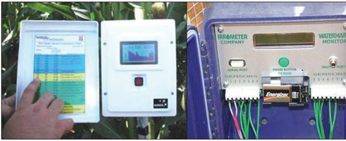
Figure 37. Hansen AM400 and Watermark datalogger for Watermark sensors.
