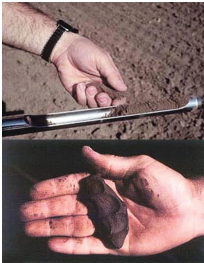
Figure 31. Sampling and evaluation techniques for the feel method of soil water monitoring.
