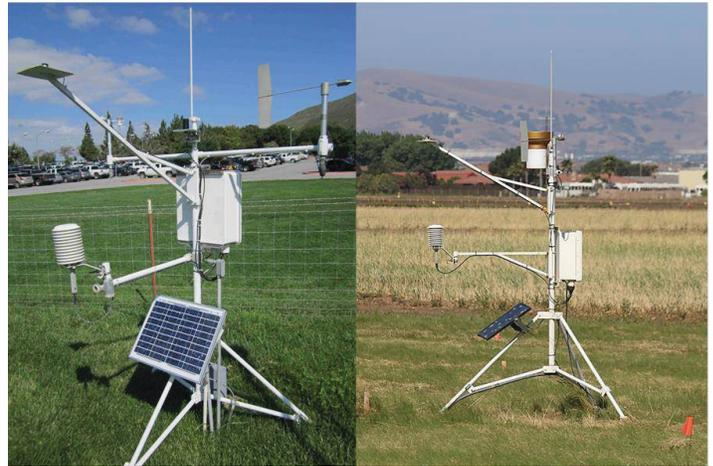
Figure 94. Weather stations for computing reference ET.
