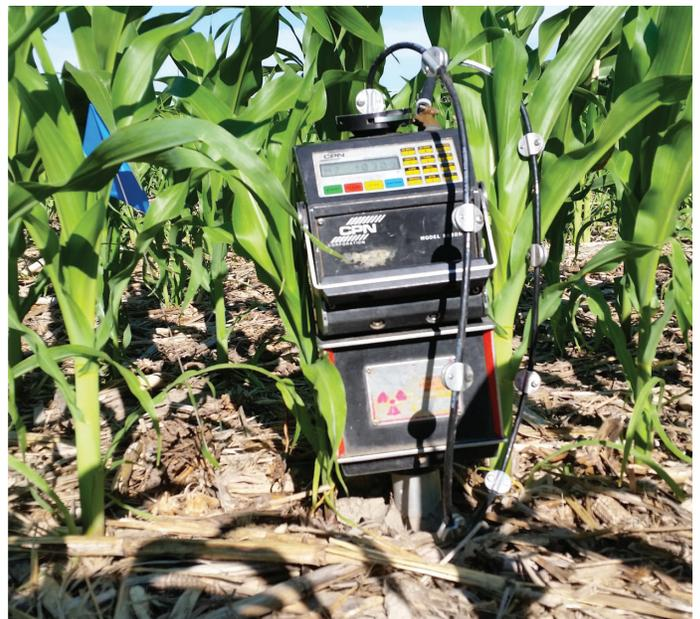
Figure 2. Installation of an access tube (A), standard count measurement (B), and in-season field measurement of a CPN 503DR Hydroprobe™ (neutron gauge) (C).
