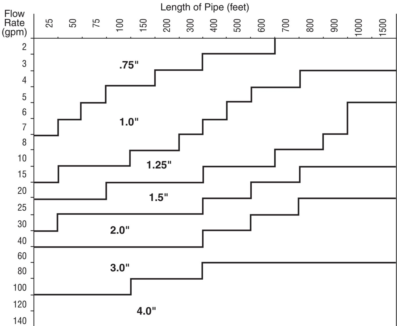
**Figure 1.** Frictional loss of water flow caused by friction between the flowing water and the internal pipe surface.
