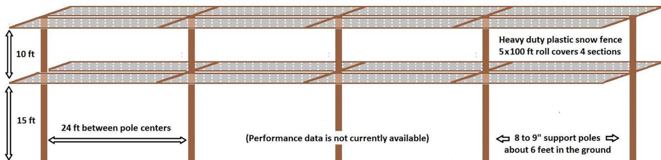
Figure 3. The USMARC high-rise shade design.
