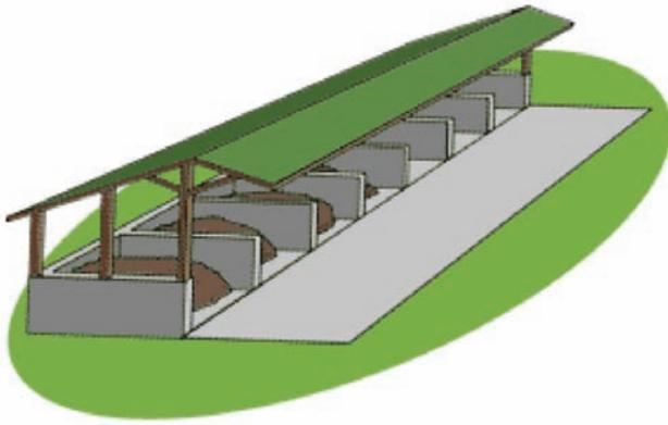
Figure 3. Roofed composting unit (high investment option).
